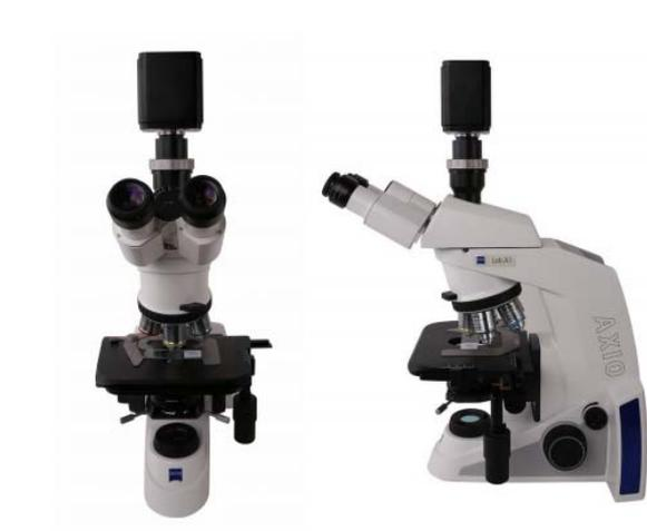
Figure 6-2 XCAM4K Camera and Zeiss Microscope
