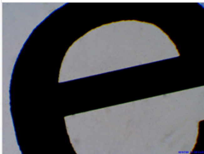
21.Letter"e" W.M. The edge color is caused by the objective lens' color aberration
