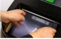
Press forward button until film appears at device front.
