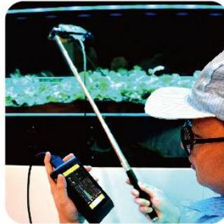
Application 2: Sensor head can be used with a selfie stick and camera tripod.
