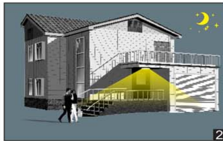
With insufficient ambient light, the sensor switches on the lamp when motion is detected.
