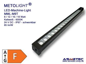
The built-in high-performance LEDs type 3030 have an efficiency of 85 lm / W at CRI Ra> 80 (optionally CRI Ra 90 available), designed for extra long life time. The LEDs are protected by a clear, break-proof front glass. The light angle is about 36° provided by special lenses to achieve perfect directed light.
