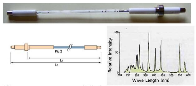
Brightness Lamp position Light spectrum 35000 cd/cm<sup>2</sup> horizontal 365 nm / 15 mW/cm<sup>2</sup>
