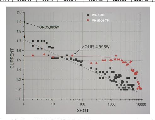
Compared to original lamp METOLIGHT MH-5000-TPI offers a constant power and current for more than 1000 shots and offers a more constant and longer life time than the original lamp which rapidly looses power after the first shot and is below MH-5000-TPI after about 15 shots.
