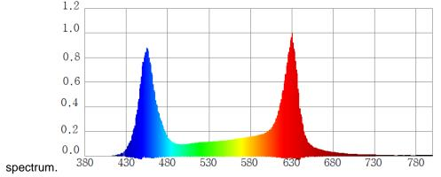
**METO***LIGHT*<sup>®</sup> **MEAT-P**: Here, the pink light is generated directly from individual specially coated SMD LED diodes. The color intensity is lower than in the RBW variant and optimal for light-colored meat, e.g. Pork suitable. In comparison to the RGW variant, the red component in the light spectrum is significantly reduced and shallower.
