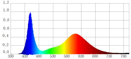
**METO***LIGHT*<sup>®</sup> **MEAT-TR**: As with variant P, the pink light is produced from specially coated SMD LEDs, whereby the colouring is somewhat lower. This colour is ideal for light poultry meat.
