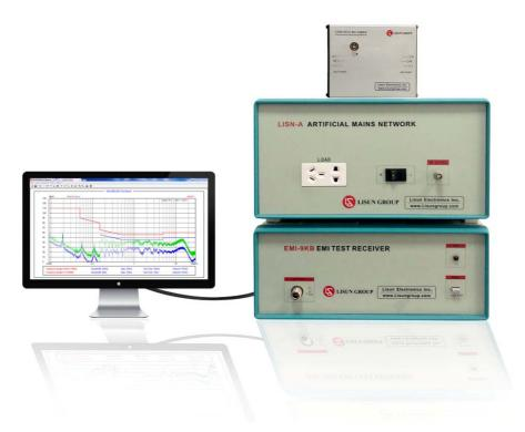
The EMI-9KA/EMI-9KB System were used to test the 9K-300MHz Electro Magnetic Interference for **Lighting Luminaries**, **Mobile and Networks**, **Automotive Electronics and Home Applications**
