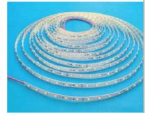
The LED strips in this series have their own CC control for each LED segment of 96 mm, which compensates for the voltage drop over the entire length. This ensures that all LEDs light up with the same brightness from the beginning to the end of the strip. The brightness of the LED strips can be adjusted using suitable low-voltage dimmers in the 24-volt range. We recommend to connect each LED-strip of 5 m length directly to the LED power driver.
