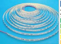
The LED strips in this series have their own CC control for each LED segment of 96 mm, which compensates for the voltage drop over the entire length. This ensures that all LEDs light up with the same brightness from the beginning to the end of the strip. The brightness of the LED strips can be adjusted using suitable low-voltage dimmers in the 24-volt range. We recommend to connect each LED-strip of 5 m length directly to the LED power driver.
