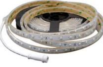
The LED strips are embedded in glass clear silicon tube reach IP class IP67 – water proof. The LED strips in this series have their own CC control for each LED segment of 5.08 cm, which compensates for the voltage drop over the entire length. This ensures that all LEDs light up with the same brightness from the beginning to the end of the strip. The brightness of the LED strips can be adjusted using suitable low-voltage dimmers in the 24-volt range.
