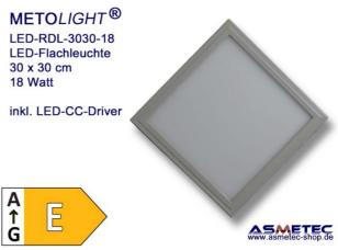
surface. The sturdy aluminum frame is matt white as standard, but can be manufactured in many RAL colors on request, taking minimum delivery quantities into account. It also serves as a heat sink for the LEDs. Even in continuous operation, the luminaire does not get warmer than approx. 35  $^{\circ}$  C. The panel luminaire corresponds to LM 78 and LM 79 with an efficiency of 120 lm / W
