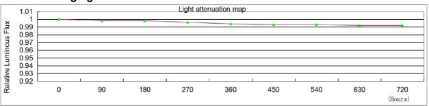
Based on the data obtained from an accelerated aging test over 720 hours with extreme temperature fluctuations, an average operating time of approx. 40,000 hours can be expected. The loss of light is less than 1% per 1000 hours
